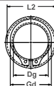
Clearance Diameter & Gaging Diameter Released in Groove.
