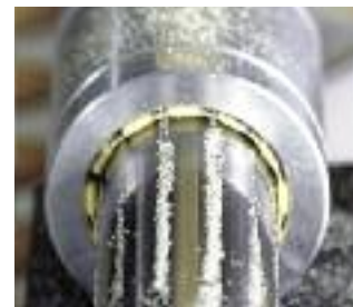
High wear resistance: plain bearing in contact with sand
