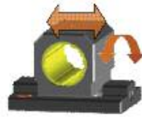
The self-aligning DryLin® R bearings of the 06 LL design series can compensate parallelism errors up to ± .12" (3mm).
