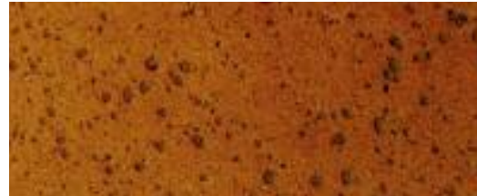
Base plastics without reinforcing materials with solid lubricants, magnified 200 times, dyed.
