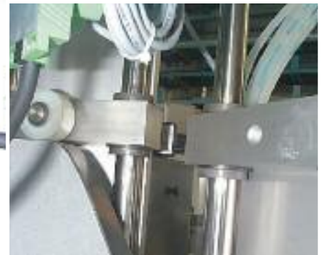
This application, a rotary transfer machine, seals champagne bottles with corks, aluminum caps and wire braid. The fact that the DryLin® guide systems are lubricant free is important in the food processing and packaging industries, additional benefits include resistance to chemicals and cleaning.
