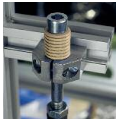
Polysorb Disc Springs in a fatigue test
