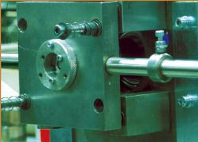
This is an example of friction and abrasion measurement in a rotation test.
