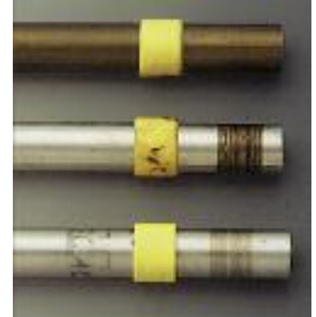
Wear experiments with aluminum shafts
