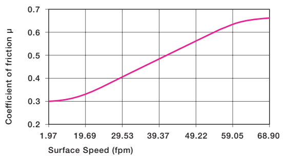
Coefficient of friction of iglide® M250 as a result of the surface speed; p = 108 psi
