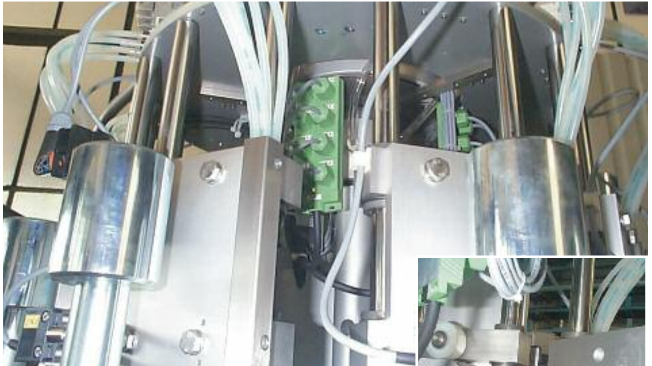
This application, a rotary transfer machine, seals champagne bottles with corks, aluminum caps and wire braid. The fact that the DryLin® guide systems are lubricant free is important in the food processing and packaging industries, additional benefits include resistance to chemicals and cleaning.
