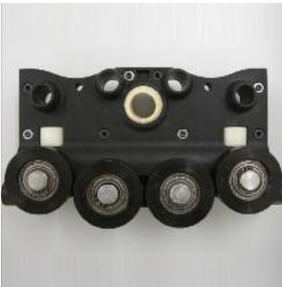
Carriage in a crane system
