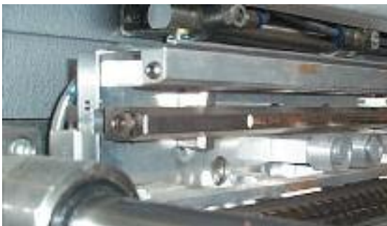
DryLin® high-temperature bearings made of iglide® T500 are used to support the sealing bar in this packaging machine. The TUM liners run without lubrication at temperatures of around 266°F, allowing a class leading output of 90 cycles/min.
