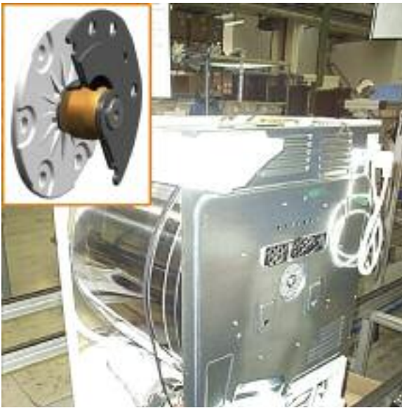
Drum bearing in a tumble dryer
