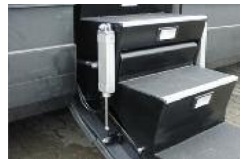
igubal® rod end bearings in the cylinder-controlled steps of an RV
