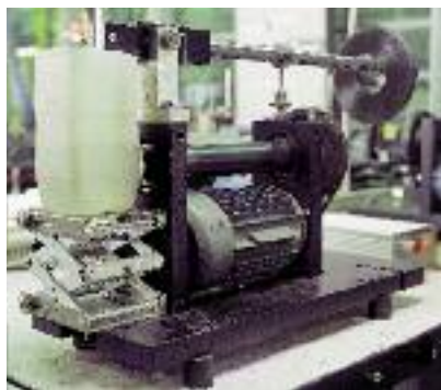
Rotational testing stand for underwater and/or chemicals
