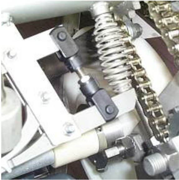
Both the housing material and the universal ball joint are made of materials that are safe in food environments
