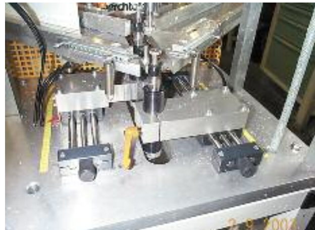
Lead screw table used to position milling heads in aluminum window manufacturing
