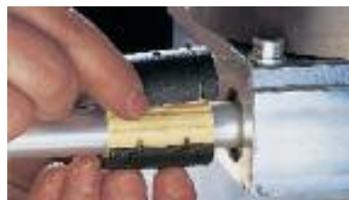
Then the adapter is fitted over the liner
