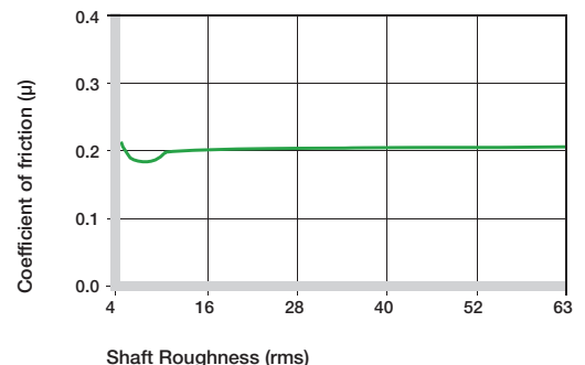
Coefficients of friction of iglide® A180 as a function of the shaft surface (1050 hard chromed)
