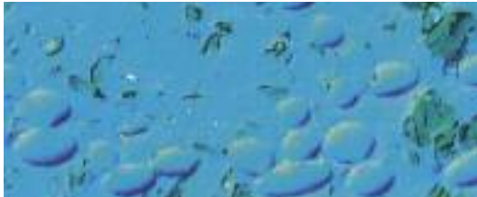
Base plastics with fibers and solid lubricants, magnified 200 times, dyed
