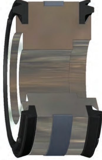
BMP installed in Piston Gland
