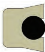
Standard PolyPak Cross-Section
