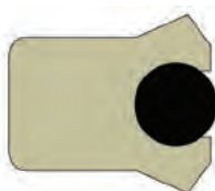
Type B PolyPak Cross-Section
