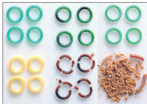
Figure 2-10. Progressive effect (hydrolysis) of high temperature water on standard urethane seals (yellow) vs. Parker Resilon® 4301 polyurethane seals (aqua).
