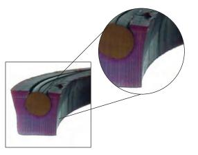
Figure 2-6. Seal wear on dynamic surface
