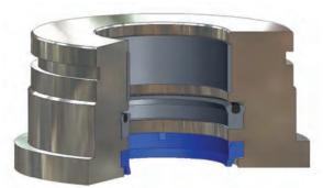
Type B PolyPak installed in Rod Gland
