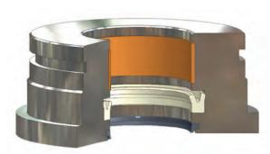
Rod sealing system comprised of PDT wear strip, B3 rod u-cup and SH959 wiper
