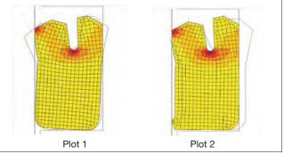
Figure 2-8. Design improvements for increased stability
