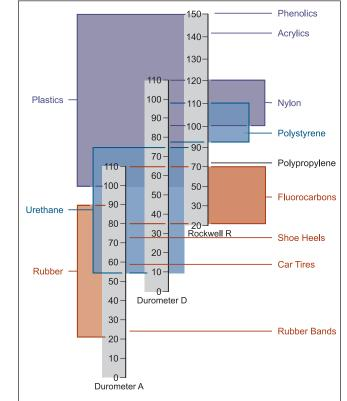
Figure 3-6. Hardness Scale Comparison Between Shore A, Shore D, and Rockwell R
