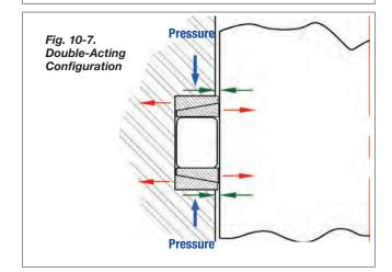
**Legend:** Blue arrow shows direction of system pressure. Red arrows show movement of wedged back-ups under pressure to bridge extrusion gap (green arrows).
