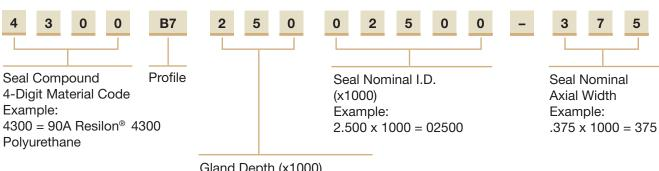
Gland Depth (x1000) or Seal Nominal Radial Cross-Section Example: .250 x 1000 = 250
