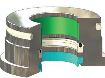
568 installed in Static Head Gland
