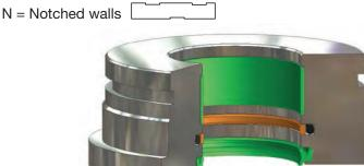
ON installed in Rod Gland
