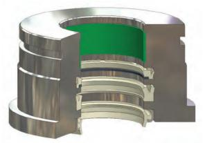
BT Installed in Rod Gland
