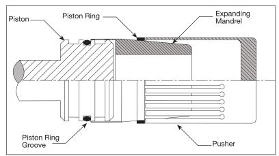
Figure 2-19. Installation of piston seal with tooling
