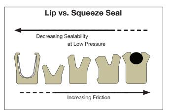
Figure 2-3. Lip seal vs. squeeze seal
