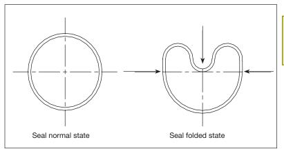
Figure 2-22. Rod seal folding
