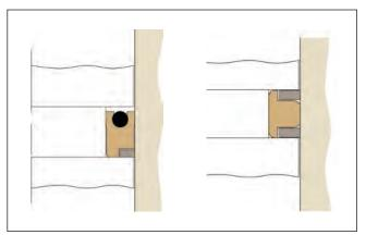
Figure 10-2. Positively-Actuated Back-up Rings
