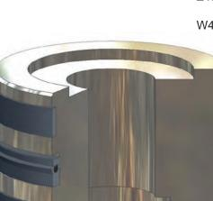
PIP installed in Piston Gland
