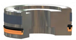
SL installed in Piston Gland
