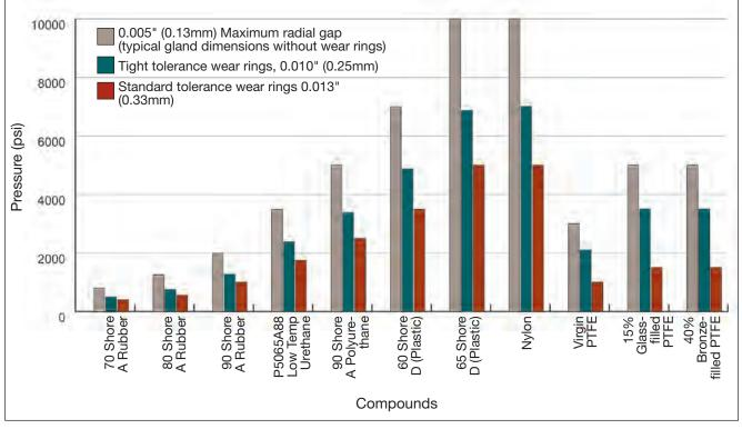
**Note:** Pressure ratings are based upon a test temperature of +160°F (+70°C). Lower temperatures will increase a material's pressure rating. Higher temperatures will decrease pressure ratings. Maximum radial gap is equal to the diametrical gap when wear rings are not used. Wear rings keep hardware concentric, but increase extrusion gaps to keep metal-to-metal contact from occurring, thereby decreasing pressure ratings when used.
