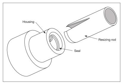
Figure 2-24. Rod seal installation
