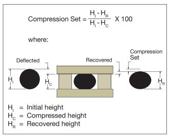
Figure 3-10. Compression set calculation
