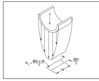
Figure 9-3: Load distribution of radial force, F, and effective load area,  $A_L$
