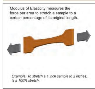
Figure 3-7. Modulus of Elasticity
