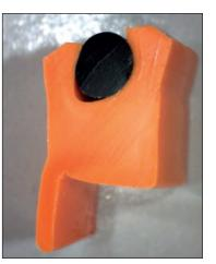
Figure 2-5. Extrusion damage
