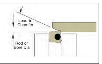
Figure 2-17. Seal installation lead-in chamfer
