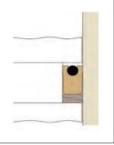
Figure 10-3. Wedged / Angled Back-up Ring
